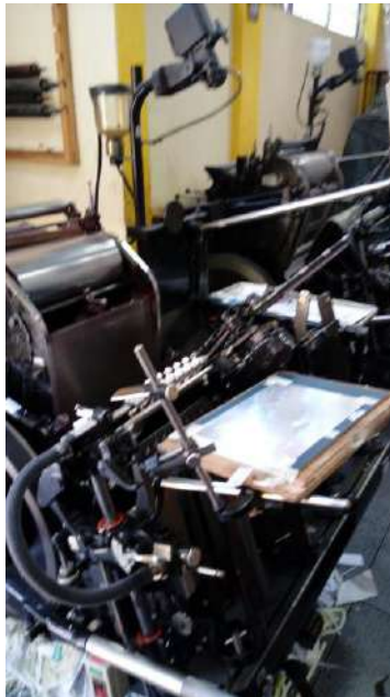
Picture 47. Heidelberg print machines adapted for braille printing
