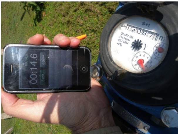
Ph. 8: Borehole BH2 flow test
